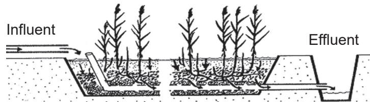
Figure B: Horizontal flow
